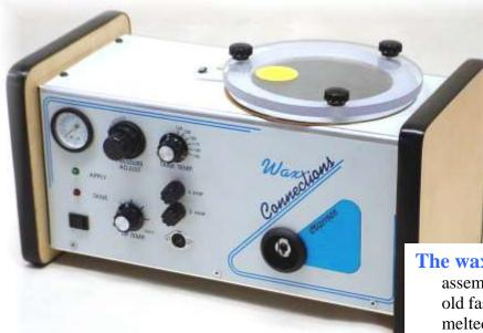
The wax applicator is a wax pattern assembly tool. Used to replace those old fashion eyedroppers and tins of melted wax, with a piece of equipment that gives the operator control.
